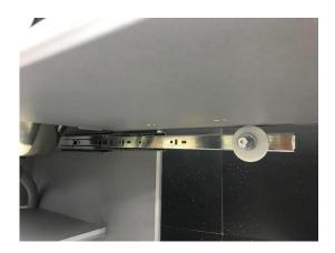
3. To store the stove push in the stove support and depending on the model of the stove, reverse the top holder and use elastic to secure the hob stand so that it doesn't stick out and catch anything. The elastic also retains the canister flap.
